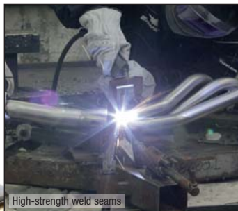
High-strength weld seams
