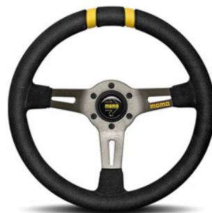
DRIFTING BLACK SUEDE, ANTHRACITE SPOKES, YELLOW LEATHER MARKERS ON THE TOP. Ø 330 mm
